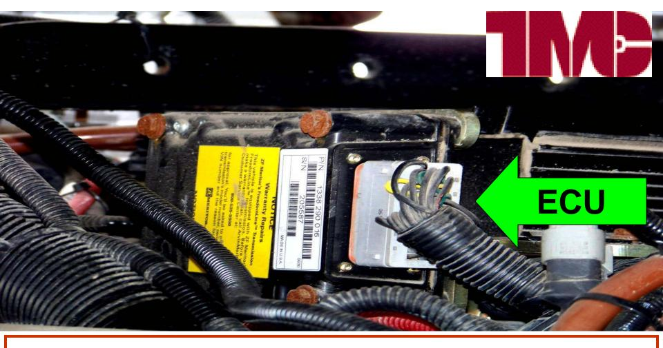
ECU lost connection with the main computer. Dealer would not provide specs needed to re-connect to network.
